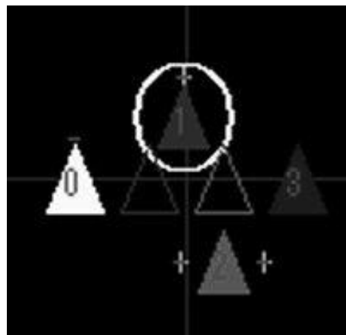
Fig. 10 “i-Con” J2ME dynamic map for (NTT DoCoMo) iappli mobile phone, featuring controllable icons in a “2.5D” application. Quasi-realtime synchronization with a CVE server motivates the use of “ghost icons,” shown as outlines, to distinguish local and session states of avatars. Workstation commands are synchronized with the mobile interface upon explicit or automatic transmission. (When a fixed-rate tariff is applied, rather than a per packet charge, our J2ME application will abandon the explicit synchronization requirement, and simply transmit reposition and narrowcasting commands as they arise. Because NTT DoCoMo can only invoke client pull, though, and not server push, explicit read will still be needed.) In this example, #0 is muted; #1 is simultaneously muted and selected and also selected for rotation (as indicated by its “halo”); and #2 is simultaneously attended and deafened.
